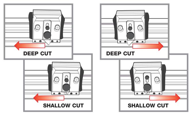
Once the blade is set move the cutting head near to the start of the cut, press down the blade holder and push or pull to make the cut. Only light finger pressure is usually required to depress the blade holder so most of your effort can be directed into pushing the blade through the material.
