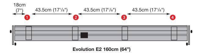
Lift the Evolution E2 cutter bar from its crate **but** <u>do not remove the clear plastic</u> <u>stretch-wrap bands</u> holding the base to the cutter bar. Place the Evolution E2 centrally on the Brackets and manoeuvre it until the base is located properly down on each of the Brackets.
