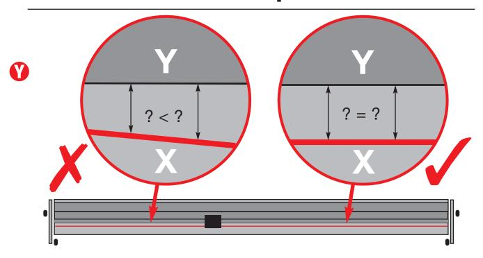
**Adjust** the straightness of the Base by adjusting the front "①" and rear "①" grub screws in the Base Fixing Brackets:
