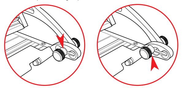
The third (furthest) position is also for cutting textile but uses a different part of the Cutting Strip should it become worn. The Cutting Strip can also be removed, turned around or flipped over to allow eight tracks to be used before the strip requires replacement. Replacement Cutting Strips are available from your Keencut agent.
