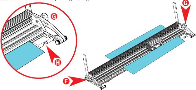
**NOTE:** If you are cutting a small piece of board place it at right hand end of the Cutter Bar against the Material Stop and place scraps of the same thickness material under the remaining bar to support it and prevent sagging.
