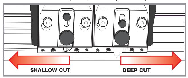
Once your blade is set move the cutting head near to the start of the cut, press down the blade holder and push or pull to take the cut. Only light finger pressure is usually required to depress the blade holder so most of your effort can be directed into pushing the blade through the material.
