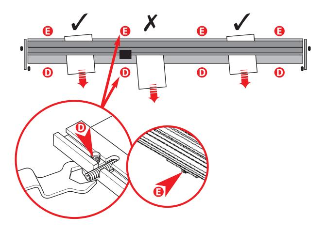
Adjust the clamping by turning the Jacking Screws "①" & "③" in the Base Fixing Brackets that are adjacent to the areas that are not clamping the paper. Turn the Jacking Screws clockwise (as you look down on them) using the wrench supplied, turn both the front and rear Jacking Screw by the same amount (to keep the Bracket level) until the paper is gripped. You may find that two or three adjacent Brackets need adjusting if you have a wide area that does not clamp.
