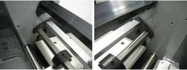
Lift the feed table off and set it on a table. Remove the six flat head screws on the front of the table shown below.
