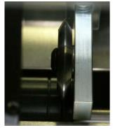
Position your score blade as desired. Scores should be made so that the blade runs on the side of the sheet that will be on the inside of the finished fold. Scores may be made on the EZ CREASER in three different ways using the different grooves on the lower score assembly.
