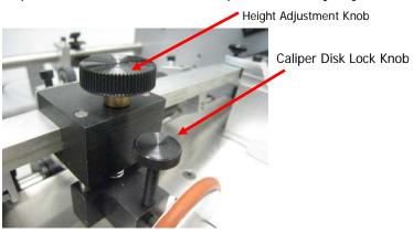
There are 2 different calipers the o-ring and the metal caliper. The metal caliper is designed to work better with heavy stock and the oring caliper is designed to work with lighter stocks. Use the oring caliper when running any multipart forms.
