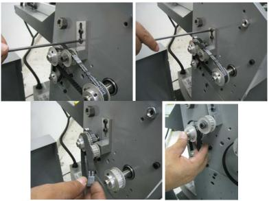
Reach in under the exit side of the machine with your right hand and slide the shaft out of the left side enough to slide the assemblies on and off the shaft.
