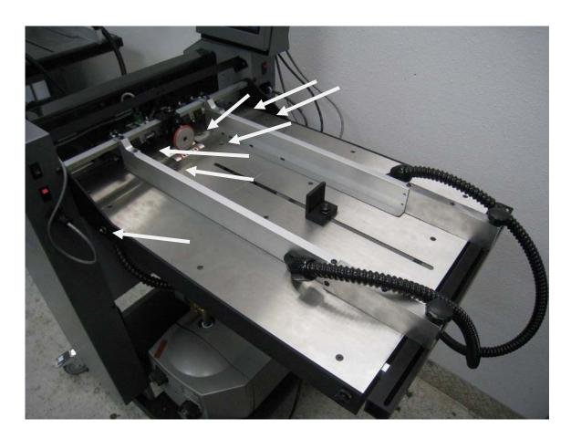
these are the bearing block screws. Also remove the vacuum pickup point adjustment knob from the operator side of the feed table. Now all the lower assemblies will drop to the table. Cut the old orings off the vacuum wheel roll the new orings on the vacuum wheel and reinstall in the reverse order.
