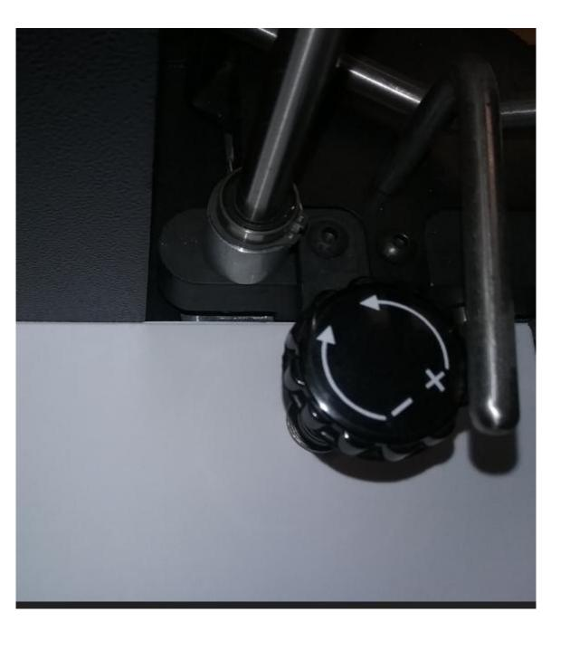
Adjust thickness of paper lift using the adjustment knob.
