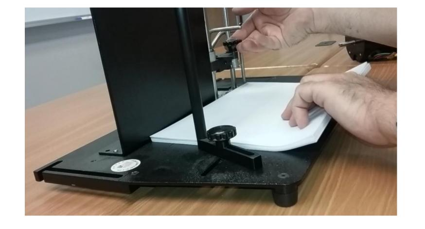
Lift up the paper weight and insert paper into the machine.
