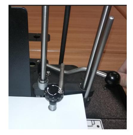
As the operating lever comes back toward the operator, the stabber goes into the paper stack and starts picking a lift of paper.
