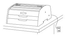
Position machine on solid surfacePlug power cord into wall outlet
