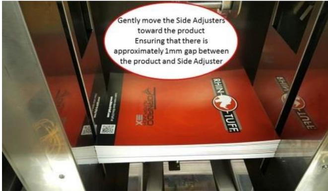
**ATTENTION!** The side adjusters are designed so that only the lever needs to be operated in order to move the side adjusters in an outward direction. To move them in an inward motion in order to ‘adjust’ on to a book, you only need to gently move the adjusters as needed. Once adjusted, the side adjuster will hold the set position throughout the entire job run or until the lever is once again operated.
