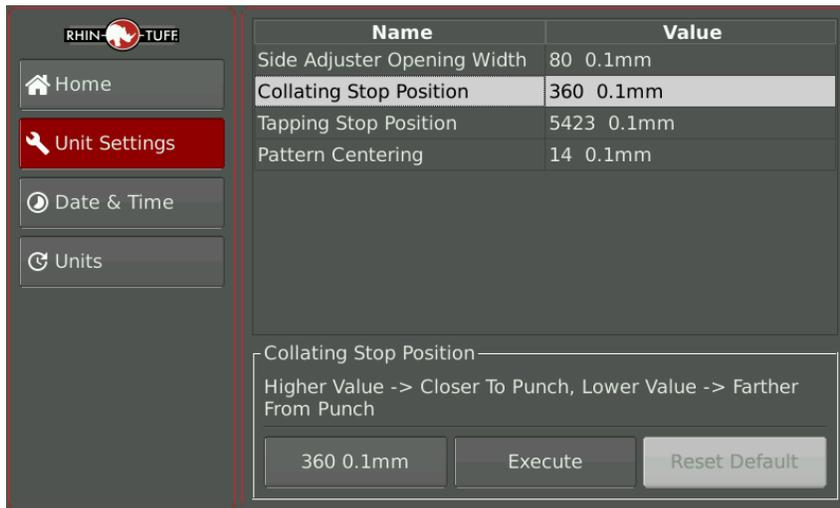
The screenshot shows the RHIN-TUFF control interface. On the left is a navigation menu with options: Home, Unit Settings (highlighted in red), Date & Time, and Units. The main area displays a table of settings:
