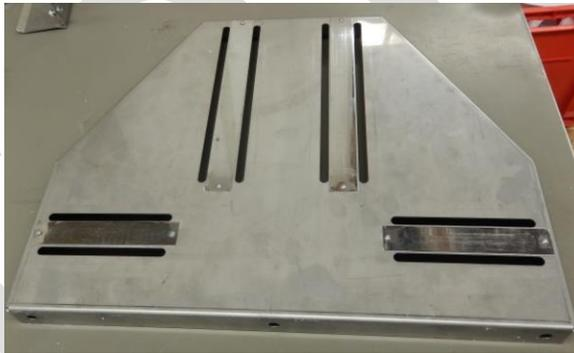
3) Install the paper guides as depicted in the picture below. They are held in place by magnets at the bottom of the guides.
