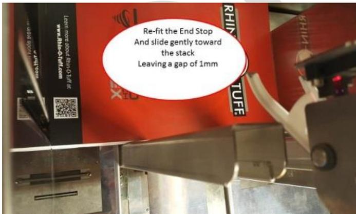
**ATTENTION!** Be aware that the media is not too tight in the hopper and there must be a gap between the media side adjusters and the leading edge adjuster. Make sure that there is a space of 1-2 mm (3/64” – 5/64”) between media and the lateral limits. Otherwise the optimal feed performance cannot be guaranteed.
