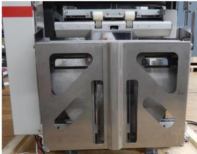
1) Attach the lift plate of the stacker to the brackets of the TAP EX with the 4 screws using Allen key 5 (Two at each side)
