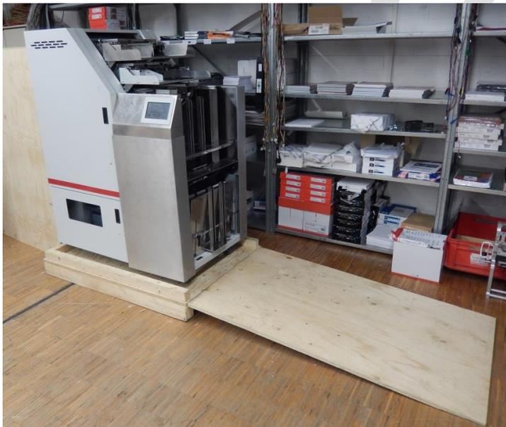
4) With the aid of a 2<sup>nd</sup> person gently roll the TAP EX down the ramp (Make sure that the brakes of the casters are released)
