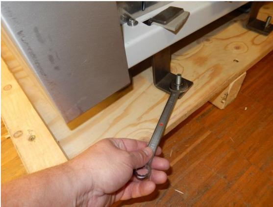
12) Remove the 4 steel brackets and the 4 bolts
