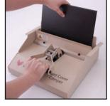
1 Immediately place Hard Cover into Crimper to crease spineand complete the binding process. Let cool in crimper before opening book.
