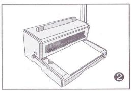
2. Fix the punching location according to the size of documents, and move out the punching selector to avoid the documents punched to break, insert the documents (upto the MAX. punching capacity) to the end, make sure the left side of documents align at punching location
