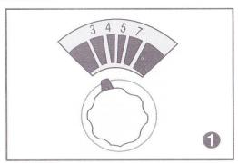
Pls select proper depth margin as per the thickness of binded documents.press and turn the depth margin adjusting knob to the needed scale(if document thickness is less than 10mm.we suggest level 3 as referred in the above picture)
