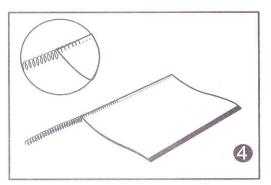
4. Select the suitable size of coil according the thickness of documents ,first put the coil 2-6 rings through the punched holes manually
