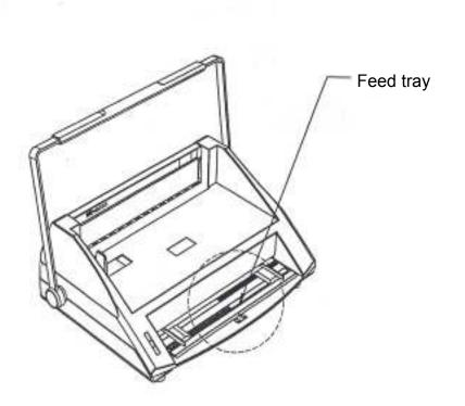
Maximum Punching Capacity: 20 sheets of 20 lb paper (75 gsm) Maximum Punching/ Binding Length: 14" (360 mm) When punching letter size documents, make sure that the center line using the red arrow on the feed tray is on "Letter". When punching legal size documents slide the red arrow to "Legal". The punched holes will not be aligned if this is not followed.
