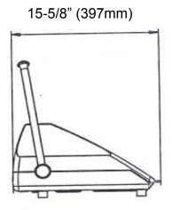
Punching Capacity: 14" (360mm) long X 1/8" (3mm) thick
