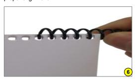
6. Manually insert the coil into the first 4 or 5 holes as shown.
