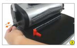
3. Adjust depth margin from 2.5mm to 6.5mm. This controls how far or how close you want the holes to be in relation to the edge of the document.
