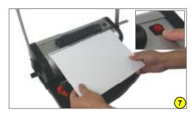
7. Press the coil inserting roller switch to the ON position (see inset) then grasp the document and gently press against the coil against the roller.
