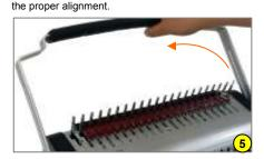
5. Select the appropriate comb element for your project then insert into the comb spreader. Grab the punch handle and push forward to open the
