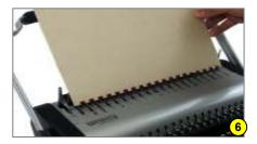
6. Insert the document into the comb making sure all teeth go through the holes then release the handle to close the comb.
