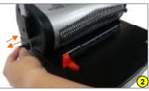
2. Adjust depth margin from 2.5mm to 6.5mm. This controls how far or how close you want the holes to be in relation to the edge of the document.
