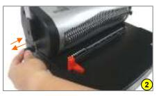
2. Adjust depth margin control from 2.5mm to 6.5mm. This controls how far or how close you want the holes to be in relation to the edge of the document.
