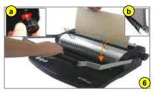
6. Adjust wire closer control to the appropriate size (see inset "a"). Insert the document into the wire closer with the wire facing downward (see inset "b") then pull the handle down to close. Remove the bound document and flip over the back cover to complete the binding process.
