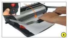
4. Adjust wire closer control to "punch" (see inset) then grasp the punch handle with 1 or 2 hands and pull down to punch holes on the document.
